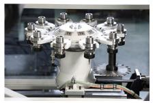
Thanks to its built-in automatic magazine with capacity for 8+1 tools, GARNET XS saves time when switching to different operations.
